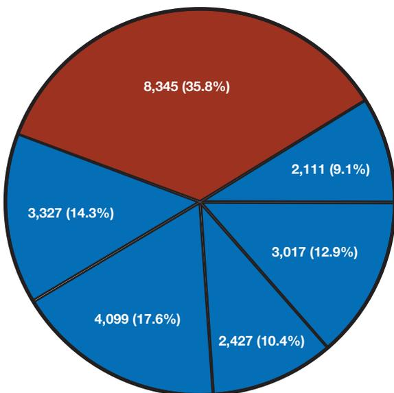
The pie chart on the left demonstrates across the six travelators that have been integrated into AEP the difference in power consumption in kWh's between the travelator that does not have a VSD compared to the five that do since the time of installation.
